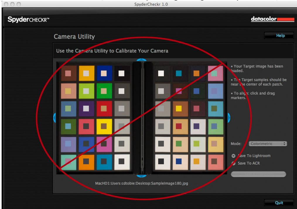
Once you have reviewed the location and orientation of the target image, click on the "Save Calibration To..." button and your calibration corrections will be calculated. You will have selected ACR or LR in advance, and will now be prompted to name your new calibration preset. This should include the name of the camera, and might include other data, such as lightsource or lens used.
