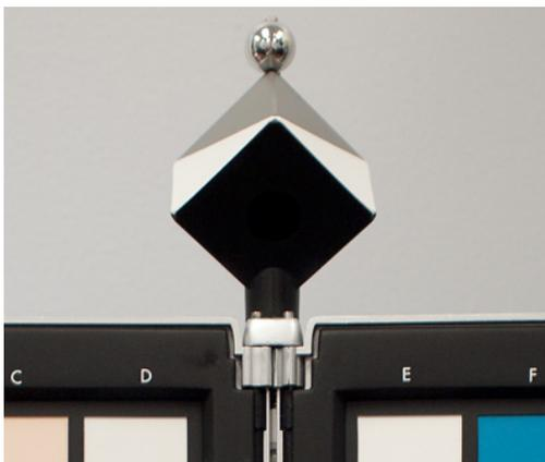
Once a camera calibration has been produced and is being used to process images from that camera in Lightroom or ACR, it is then possible to coordinate this workflow with the SpyderCube. The Cube can be used in the standard manner to determine the optimum whitepoint, exposure, black level and other basic light condition settings for a series of
