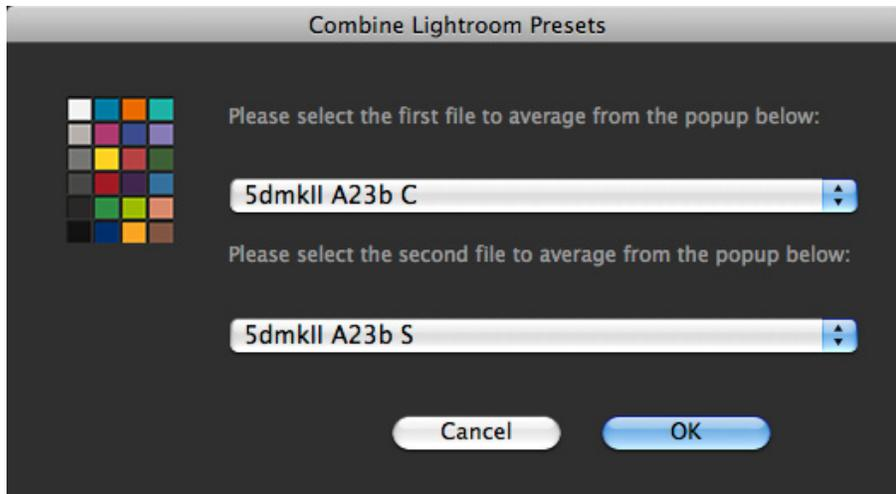
SpyderCheckr's Tools menu contains commands for creating multiple calibrations from any two existing Lightroom or ACR calibration presets. Choose any two presets built for the same camera, and a series of three new calibration presets will be created which offer increased precision for light sources between the original sources.
