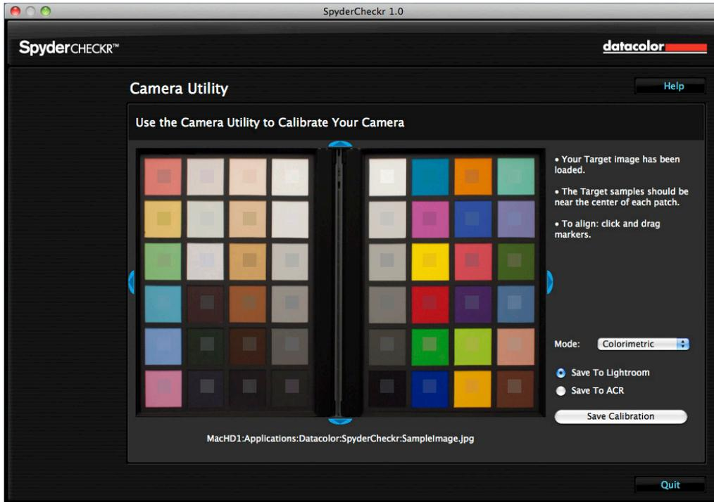
The sampling squares should already be pretty well placed within the correct patches of your Target shot if you shot and cropped appropriately. If not, you can drag on any edge or corner of the image area to adjust the fit. The colors inside the sampling squares should be a somewhat less saturated version of the patch colors. If the patch and sample colors are of different colors, check that your target image is not upside down, sideways, or inverted.
